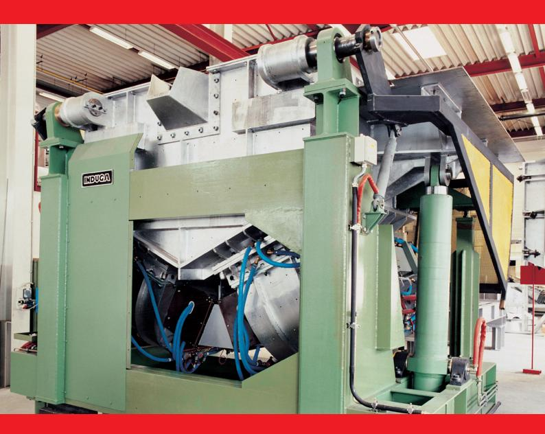
The channel type induction melting furnace with its high electrothermal efficiency, variable furnace geometry and cost effectiveness, is the preferred furnace choice for the melting of scrap or bulky materials in the non-ferrous foundry industry.
