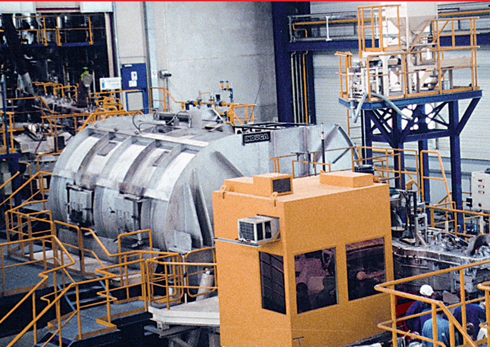
The production of semi-finished copper products in a continuous casting process makes high demands on the process and furnace concept. Besides the classical use of a gas fired shaft furnace for melting copper cathodes, the induction heated drum type furnace is an alternative way with many advantages in terms of lower oxygen and hydrogen contents, precise temperature control and higher process stability.
