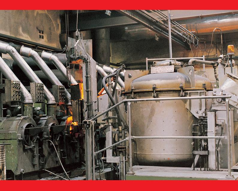
Pouring of accurate metal weights in automatic sand moulding lines, rotary casting machines or direct casting machines makes high demands on the necessary plant technology. For such applications Induga recommends the INDUMAT®, an induction heated, pressurized holding and metering furnace mounted on load cells with stopper controller.
