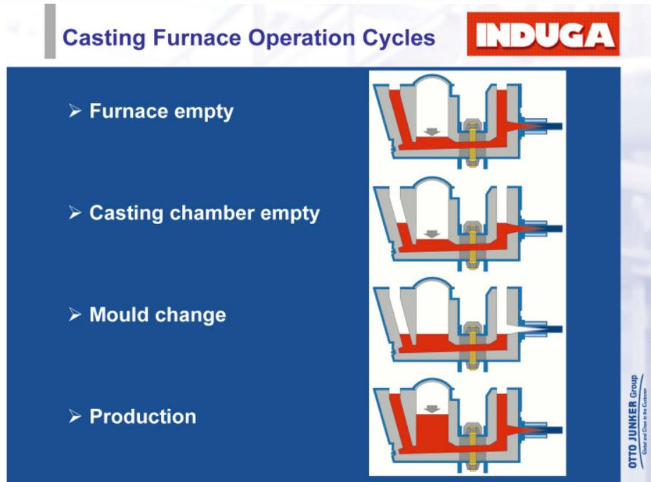
*Fig. 5: The multi-chamber pressurized casting furnace.*
