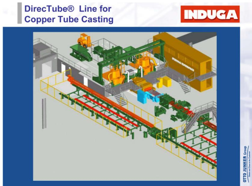
*Fig. 1: Overview of a DirecTube®-plant with charging systems, two melting furnaces, a pressurized horizontal casting furnace, withdrawal unit, saw and milling machine.*
