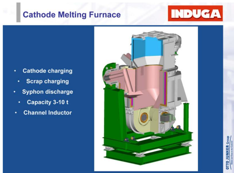
*Fig. 3: Melting Furnace for Copper Cathodes and Return Scrap.*
