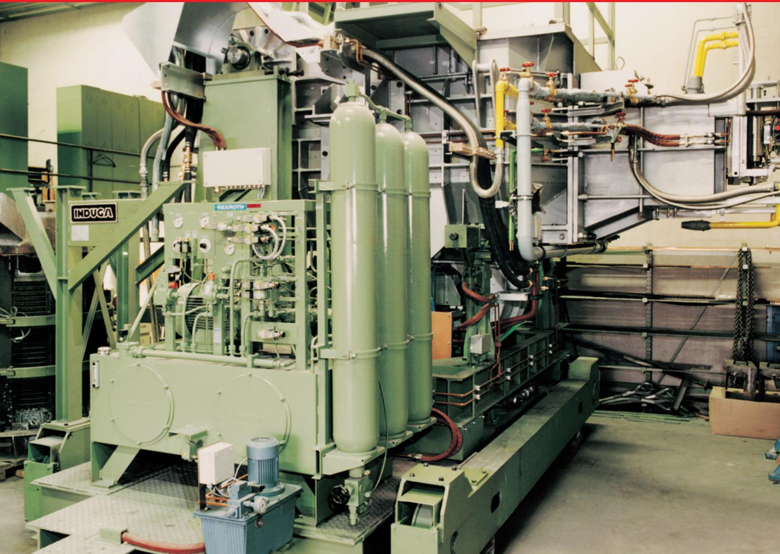
The production of vertically casted non-ferrous special alloys demands not only a highly developed continuous casting technique but also an alloying and casting furnace which is capable of supplying a homogeneous melt over the whole casting time under defined conditions with exact alloy quality and temperature control.
